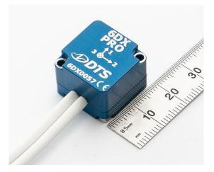
Designed for applications measuring high rates of acceleration and angular velocity, the DTS 6DX PRO packages three accelerometers and three angular rate sensors in a compact 19 x 19 x 14.5 mm package.
